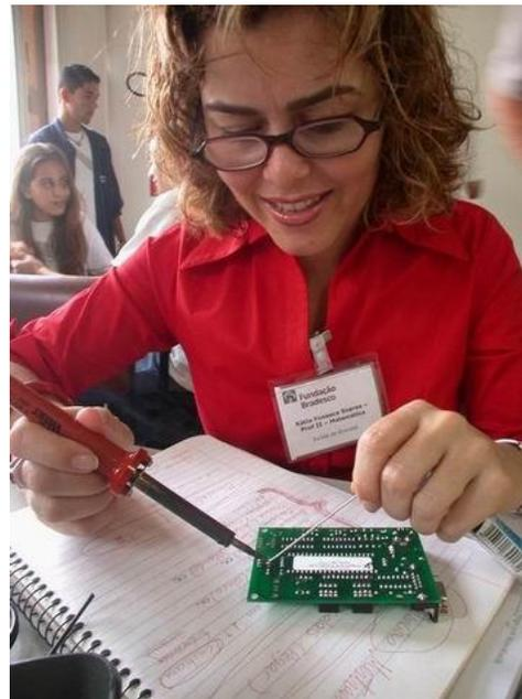
Figures 2 and 3 (left to right): Locally-Made Soil Humidity Sensor and a Teacher Adding a Memory Chip to the GoGo Board
